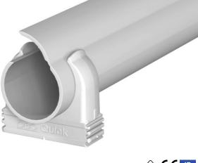
Set consisting of Quick pipe electrical installation pipes and Quick clip surfacemounted clips. For surface-mounted routing of cables in interiors and protected outdoor areas. Universal fastening on wall and ceiling. Comprises 20 m of pipe each of 2 metres in length and 60 Quick clips. Can be used in a temperature range of -25 to +60 °C.
