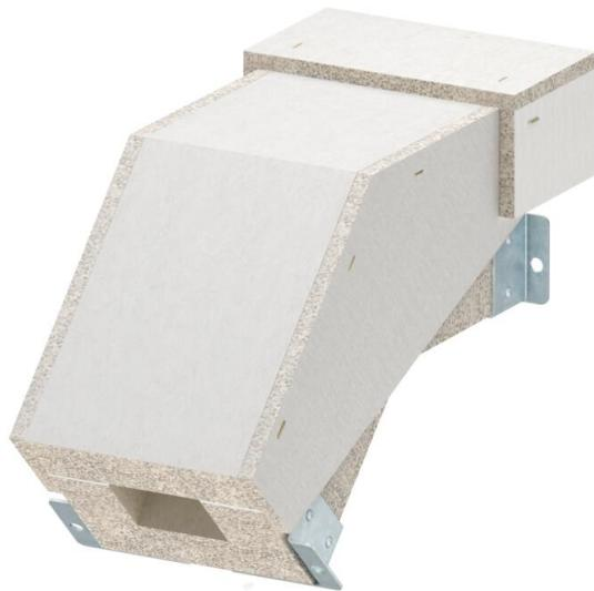
Falling vertical bend for PYROLINE® Con S fire protection duct, type BSKH09-K0506, consisting of fibreglass lightweight concrete which is resistant to water and frost for the creation of vertical changes of direction (45°) of the duct. Mounted connectors ensure quick mounting in situ, whilst loosely placed covers ensure quick inspection and reassignment.
