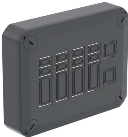
Pluggable cover for the closing of junction boxes, equipped with break-out openings for multiple-pole systems or DATA systems based on Keystone. With quick lock in cover, sealable. Halogen-free material, UV-resistant Flame-resistant to DIN EN 60695/2/11, test temperature 650 °C. Impact resistance IK07 at room temperature. Protection rating IP30
