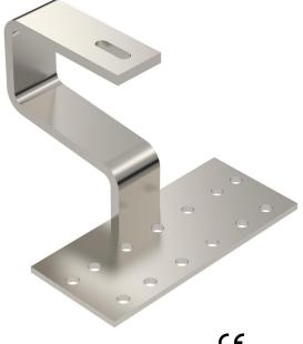
Heavy roof hook to mount photovoltaic modules on pitched roofs in combination with the TP 45 support profile. Suitable for tiled roofs. Fastening on support profile through bolt with hammer nut, type SKSHM A2. Mounting on rafters with TKS wafer-head screws.
