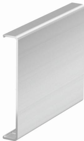
Aluminium cover, for closing Rapid GA device installation trunking and ISS service poles with a 76.5 mm system opening. The firm position of the cover and electrical contact to the lower part of the trunking and service pole is guaranteed thanks to type RKV3V locking brackets. There are 2 pre-mounted locking brackets included per delivery length (100 mm).
