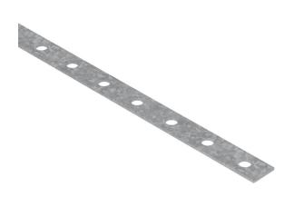
Perforated strip for cross-connecting the rear supports of pre-mounted supports type VT 10/25/30. For stiffening PV mounting systems free-standing. Fastening with screw set for perforated strip type SVLB. Fastening material not included in scope of delivery.
