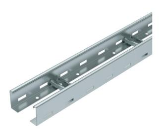
Cable ladder with a 60 mm side height with welded C30 profile rungs which are open in an upwards direction. Rolled side rail for reinforcement and as edge protection. Fastening to the bracket takes place using hold-down clamps, type LKS 40. The slot dimension of the rung is 16.5 mm and the appropriate clamp clip is type BS-H....
