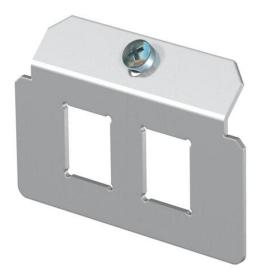
Support plate to accept two data connection modules of the following types: Brand-Rex: shielded; EKU: E-Stone; Dätwyler: KS-T, MS-K and KU-T module; R&M: Snap-In and Keystone; Rutenbeck: UM and UMflex; SETEC: MKJ, UKJ and XKJ; Siemon TERA; Telegärtner: AMJ and UMJ; 3M: CAT6 and CAT6A. Dimensions of a mounting opening in mm: 19.30 x 14.80.
