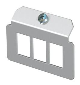
Support plate to accept three data connection modules of the following types: AMP TYCO: SL series 110Connect and Toolless, AMP-Twist; Brand-Rex: unshielded; GG45; TKM RJ MOD; Nexans: LANmark with Adapter Clip. Dimensions of a mounting opening in mm: 20.10 x 14.80.
