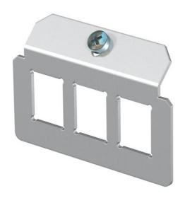
Support plate to accept three data connection modules of the following types: Brand-Rex: shielded; EKU: E-Stone; Dätwyler: KS-T, MS-K and KU-T module; R&M: Snap-In and Keystone; Rutenbeck: UM and UMflex; SETEC: UKJ and XKJ; Siemon TERA; Telegärtner: AMJ and UMJ; 3M: CAT6 and CAT6A. Dimensions of a mounting opening in mm: 19.30 x 14.80.
