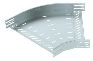
45° bend for the creation of a horizontal branch, fitting for lock and screw-on cable trays of side height 60 mm. Screwless mounting with double clamps or screw connection with FRS truss-head screws and M6 combination nuts. Can be used in indoor areas. Fastening material must be ordered separately.
