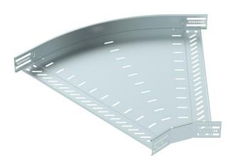
45° bend for the creation of a horizontal branch, fitting for lock and screw-on cable trays of side height 60 mm. Screwless mounting with double clamps or screw connection with FRS truss-head screws and M6 combination nuts. Can be used in indoor areas. Fastening material must be ordered separately.
