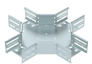
Cross-over for the creation of a horizontal branch, fitting for lock and screw-on cable trays of side height 60 mm. Screwless mounting with double clamps or screw connection with FRS truss-head screws and M6 combination nuts. Can be used in indoor areas. Fastening material must be ordered separately.
