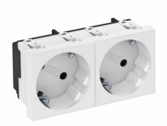
Protective contact socket, double 33°, with increased touch protection, with screwless terminals, 2-pin, 16 A, 250 V~, with connection terminals to IEC 60884-1
