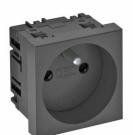
Socket with earthing pin, single 0°, with increased touch protection, with screwless terminals, 2-pin, 16 A, 250 V~, with connection terminals to IEC 60884-1.
