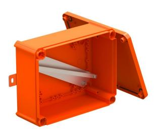
Unequipped, closed connection or junction box for free termination with ceramic terminals and cable glands. Dimension A states the available support rail length for the wiring terminals. Sufficiently large wiring compartment through diagonally arranged support rail. Fastening on easily accessible external flaps made of stainless steel. Approved for cable systems that maintain the electrical function according to DIN 4102 Part 12 with the classes E30, E60 and E90.
