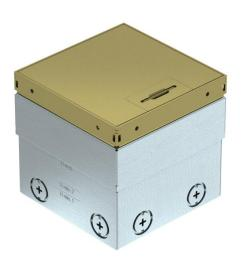
Square floor socket for use in dry-care cavity and screed floors. Installation housing with pre-marked insertion openings for pipes (M20/M25). Cover adjustable to top edge of floor covering using four height-adjustment supports. The minimum installation depth is 100 mm, the height-adjustment range 35 mm.Frame and cover made of brass and visible in the floor covering. Empty housing for up to 2 Modul 45® devices in the mounting support and 2 data sockets in the optional data technology support.
